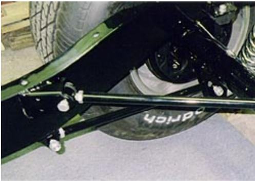
Various methods are available to adjust for proper pinion angle. On a parallel leaf spring, wedge shaped shims can be added between the spring and spring pad. On triangulated 4-link, such as this, the upper and lower links can be lengthened or shortened as required.
