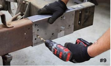
\* With the Template in place, using a 3/8" drill bit, drill the NON-underlined holes that correspond with your year range (72 for '67-'72, 66 for '63-'66) as shown above in #9 on a 67-72 frame.
