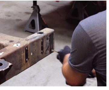
Next, you'll be removing the rear cab mounts and forward most bed mounts from the frame. Using an air chisel (or alternatively a grinder), cut off the heads of the rivets holding the rear cab mounts and forward bed mounts to the frame. Once you have removed the heads of the rivets, use a punch to drive the rivets out of the mounts and the frame (as shown below).
