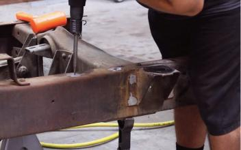
Now that BOTH sides have been drilled, cut-off and the bed and cab mounts have been removed, it's time to relocate the cab mounts. You'll be using the center section of the template that was set aside earlier, but first the Template needs to be prepped.
